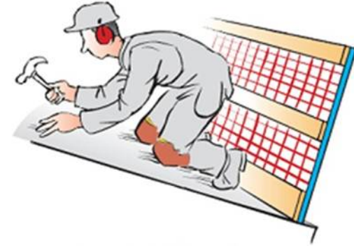
Guardrail at roofing works
